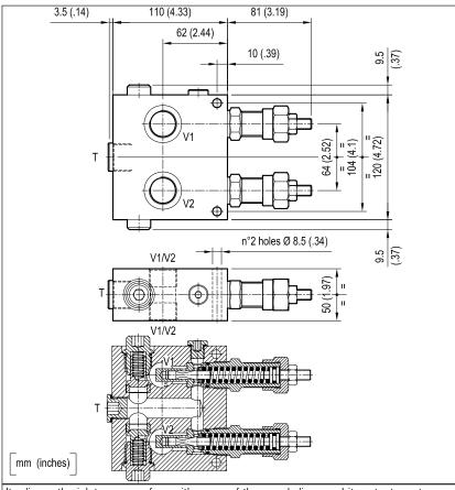
It relieves the inlet pressure from either one of the supply lines and it protects motors or hydraulic actuators from shocks or pressure surges induced by changes in direction or by sudden stops. The dual relief is of the cross over type, and exhausted oil is transferred to the other line (from V1 into V2 and vice-versa) to prevent cavitation. An extra tank port (T), with 2 checks, allows to make up for any drain or exhausted flow and ensures that the motor is always full.
