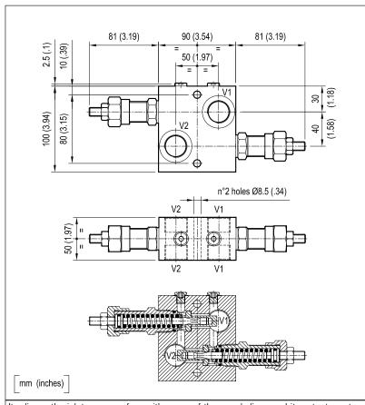
It relieves the inlet pressure from either one of the supply lines and it protects motors or hydraulic actuators from shocks or pressure surges induced by changes in direction or by sudden stops. The dual relief is of the cross over type, and exhausted oil is transferred to the other line (from V1 into V2 and vice-versa), without the necessity of a separate tank line: this feature also prevents cavitation when used in conjunction with closed centre directional valve.
