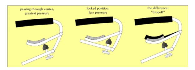
The roller mechanism equalizes the dropoff across the full range of the capo.
