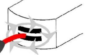
(c) Slowly rotate the demagnetizer tip in a circular motion while slowly pulling away until a distance of 12". Once complete, unplug demagnetizer from the power source.
