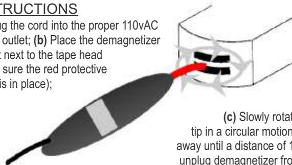
(c) Slowly rotate the demagnetizer tip in a circular motion while slowly pulling away until a distance of 12". Once complete, unplug demagnetizer from the power source.
