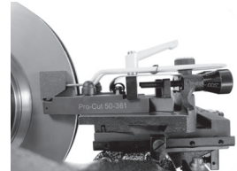
The chip deflector reduces vibration and should be used on EVERY cut.
