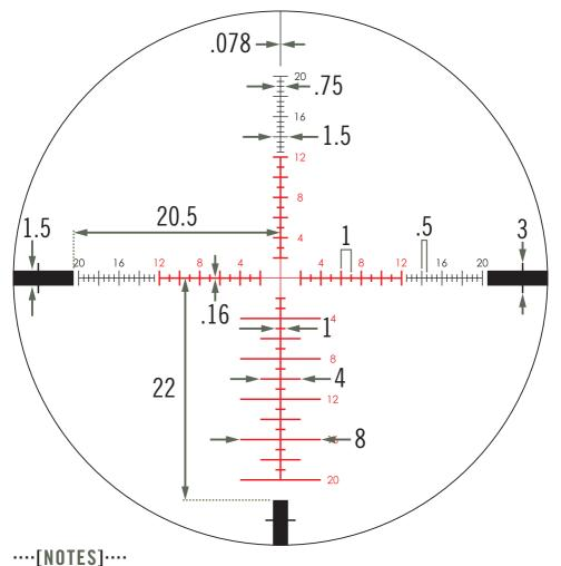
Subtensions are measured in MOA and correspond to the highest magnification.  $\emptyset$ =Diameter
