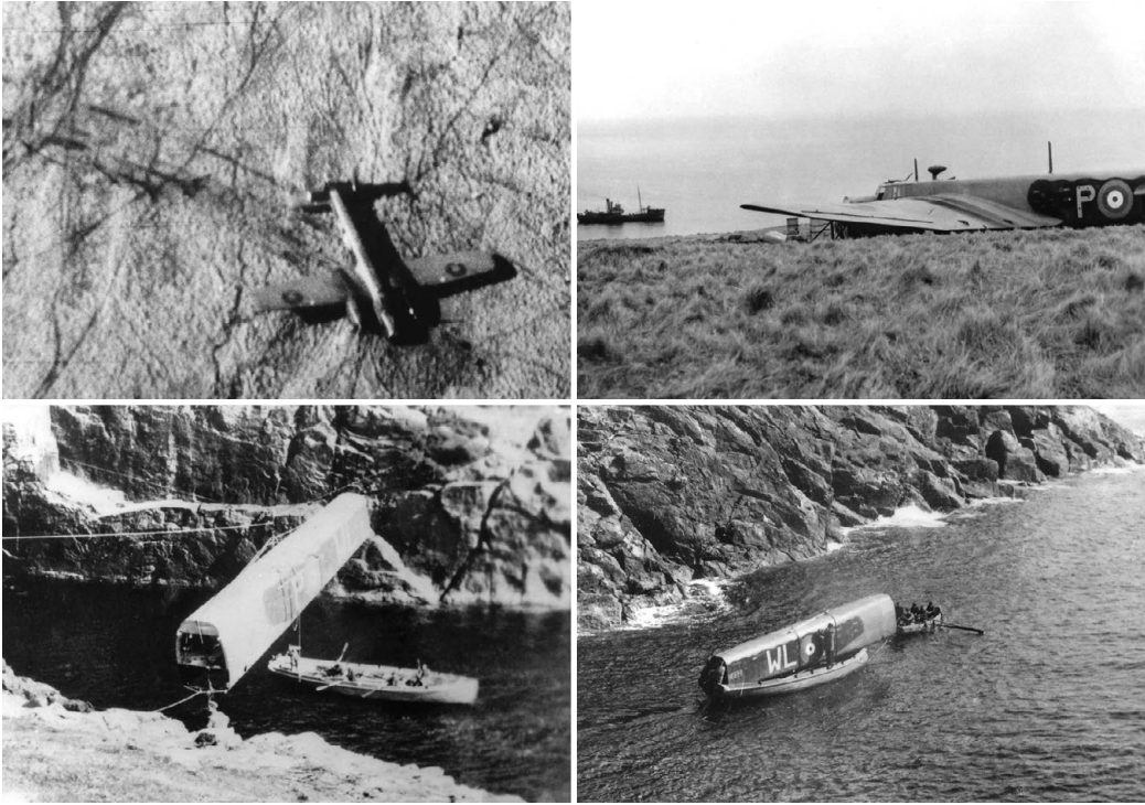
Plate 7. The RAF Whitley bomber on North Rona after its successful emergency landing. The plane was dismantled and taken off the island. It was reassembled and flew again operationally. © 'After the Battle'
