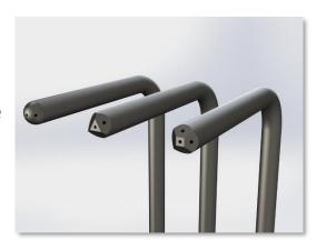
Multi-hole probes allow measurement of the full 3D flow velocity vector. We have developed sintered solutions that both reduce the probe head size and increase the operating envelope. We can produce a 5 hole probe with a diameter as small as 6mm.
