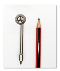
Our patented designs measure wind speed, pitch and yaw angle with improved stability over traditional multi-hole probes, and directly measure total pressure which can be used as a reference for scanners.
