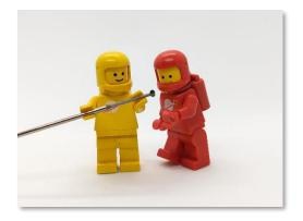
Through our ground-breaking work on additive manufacturing methods, we have developed techniques that allow us to build our tiny Micro-Kiel probes with a head diameter as small as 1.6mm. This allows accurate measurement of flows with minimal intrusion.
