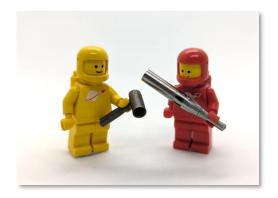
Kiel probes are designed to measure the total pressure with insensitivity to wind yaw and pitch angle. Used in a wide range of applications, they have become particularly popular used in arrays known as "rakes" in Formula One.
