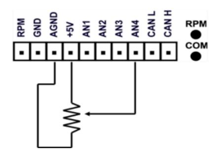
Connecting to a potentiometer already installed on a car, such as a throttle potentiometer, would only require the output signal from the pot and the earth to be connected to the MICIN01.
