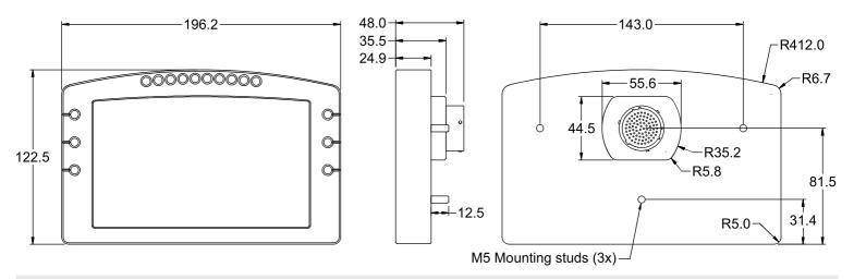
Note: Do not remove any part of the casing. The case provides electromagnetic screening to avoid interference with other equipment, and is also essential for thermal management. Thermal management may be compromised if mounted in a confined space, refer to the operating temperature specifications.
