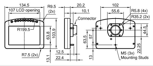
Note: Do not remove any part of the casing. The case provides electromagnetic screening to avoid interference with other equipment, and is also essential for thermal management. Thermal management may be compromised if mounted in a confined space, refer to the operating temperature specifications.
