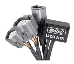
MoTeC's LTCD NTK (Lambda To CAN) is the dual sensor version of the LTC NTK. It monitors, controls and diagnoses two NTK Lambda sensors, transmitting Lambda readings on a CAN bus. When using Dual LTCs or a mix of singular and Dual LTCs, up to 32 Lambda sensors can be configured on a single CAN bus for simultaneous monitoring by an ECU or logging device.
