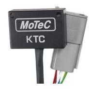
The KTC (K-Line to CAN) adaptor converts CAN data to ISO 9141 K-Line data with specific formats to facilitate communication between MoTeC 'hundred series' ECUs and existing dashboards in Yamaha and Kawasaki Jet Skis.
