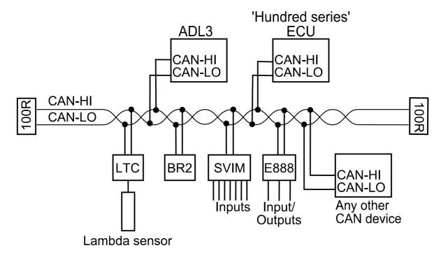
The SVIM is powered from the vehicle battery and connected to the Data Logger via the CAN bus.
