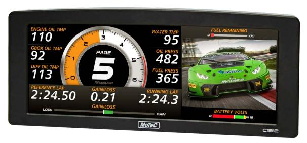
The C1812 comes standard as a combined 12" full colour display, powerful control device and fully programmable data logger with 250 MB internal memory. Optional USB Logging provides additional data capacity and flexibility, and also upgrades the internal memory to 500 MB.
