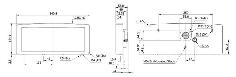
Note: Do not remove any part of the casing. The case provides electromagnetic screening to avoid interference with other equipment, and is also essential for thermal management. Thermal management may be compromised if mounted in a confined space, refer to the operating specifications.
