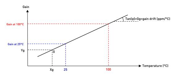
The values {Xg; Yg; Gg} fully define the gain compensation curve. Please refer to chapter 7.2.4.3 to know how to configure the gain settings.
