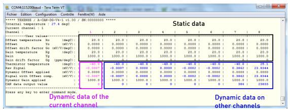
Note: In view mode, the CAN data output frequency is set to 1Hz in order to have the best filtering features for display and calibration. The frequency automatically goes back to its configured value when leaving this mode.
