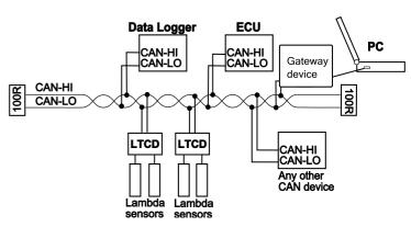
For information on wiring a CAN bus with several LTCs and any number of other CAN devices (as in the example), refer to the relevant device manual.
