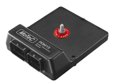
MoTeC's 15 output Power Distribution Module is designed to provide electronically switched power to various electrical systems in the vehicle such as motors, lights, solenoids, and electronic devices such as ECUs and data acquisition systems.
