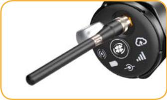
Make sure the antenna is properly attached before proceeding.
