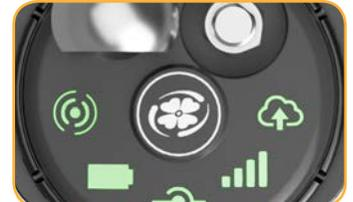
Press the button. All LEDs turn on. Then each LED changes color according to device status.
