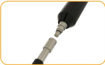
Disconnect the instrument from VuLink. Attach another. Press the button.
