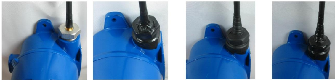
Figure 65 Water-proofing Antenna Connections
