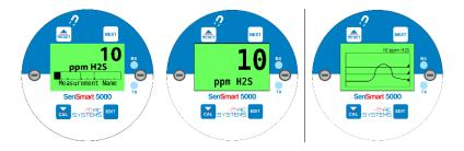
Figure 9 Universal Gas Detector Data Display Screens
