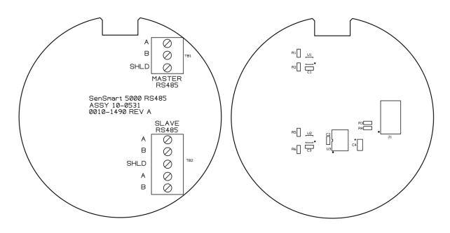
Figure 18 10-0531 Modbus Board
