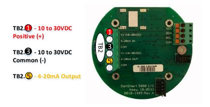
Figure 3 SenSmart 5000 Wiring
