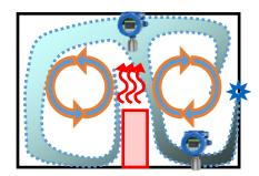
Vapor density of a gas determines if it will rise or fall in air when there are no significant currents. Lighter than air gases should have the detector mounted 12 to 18 inches (30 to 45 cm) above the potential gas leak, and heavier than air gases should be this distance below the potential gas leak.
