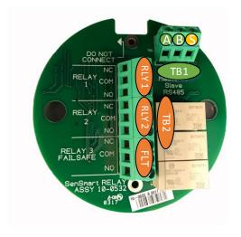
Figure 5 SenSmart 5000 Relay Option Wiring
