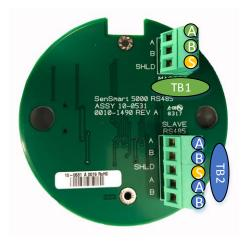
Figure 4 SenSmart 5000 Modbus Option Wiring
