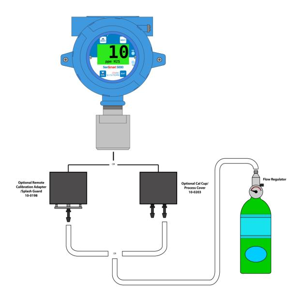
Figure 12 Calibration Diagram
