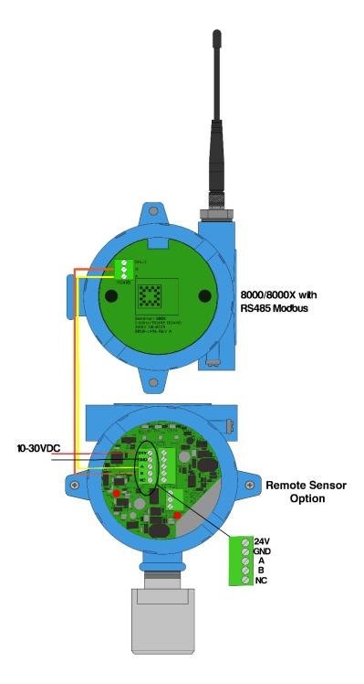
Figure 7 Wireless Remote Sensor Option
