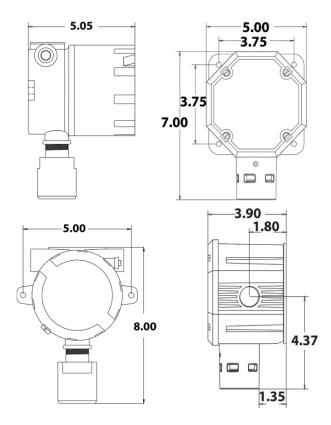
Figure 1 Mounting Dimensions
