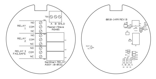
Figure 21 10-0532 Modbus/Relay Board
