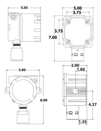
Figure 15 Mounting Dimensions
