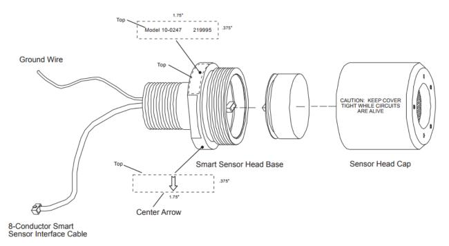
Figure 8 Stainless Steel Sensor Head
