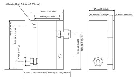
NOTE: The assembly is shown with ¼ inch OD tube fittings. The dimension across the tube fittings will vary for all other size fittings.
