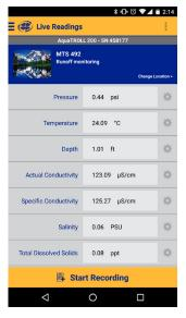
Use the VuSitu Mobile App to access and manage data on your Android<sup>™</sup> smartphone or tablet. Intuitive, free mobile app is an all-inone software package that provides autoconfiguration, simplified calibration, guided log setup, directed data anaysis, and automated report creation. Tag data with site photos and GPS coordinates. View results in the field and email data on the spot. Download through the Google Play Store.
