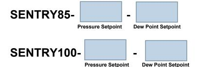
For Example: **SENTRY85-75PSIG – 10F** would be a Sentry 85 unit with a low pressure alarm set to 75 psig and the high dew point alarm set to +10°F.
