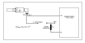
**Note**: the maximum value for Rs in this circuit can be calculated by the formula:
