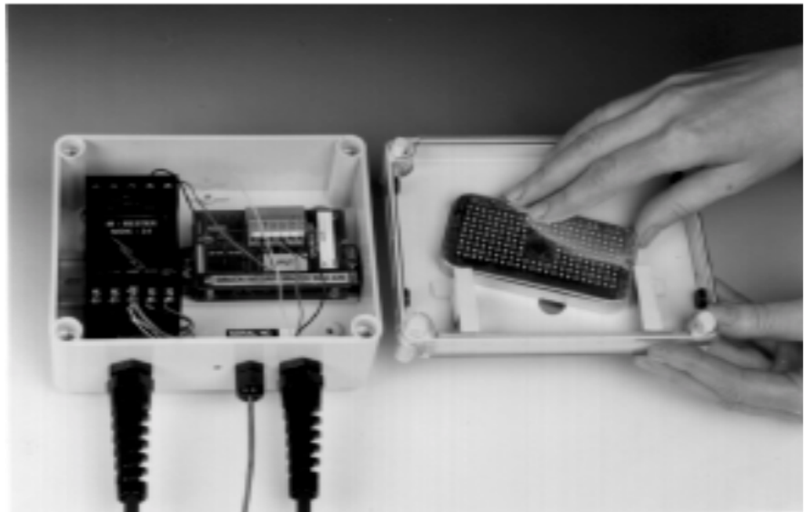
SCU 220 with cover removed showing desiccant module; shown here with MDK-LC lightning arrester
