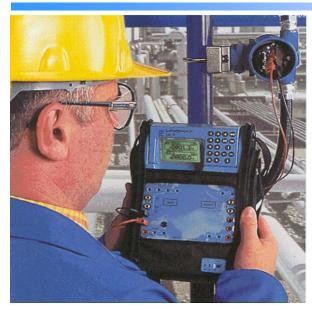
Direct connection of thermocouple compensation wires eliminates the need for special connectors. The cold junction temperature is continuously monitored and compensated for, even under the transient conditions experienced by a field calibrator. This is the most reliable and accurate cold junction compensation method found in a portable field calibrator.
