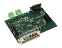
This card provides an XCi device with the ability to control/log In-Situ and 3rd party SDI-12 compliant sensors.
