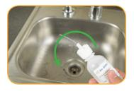
Lightly shake the bottle of reference filling solution and turn upside down to mix.
