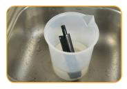
Soak sensor for a minimum of two hours in 140 mg/L nitrate as N standard or the highest standard you plan to use during calibration.
