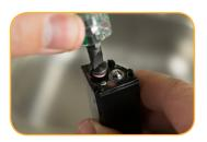
Overfill slightly. Reinstall reference juntion cap and tighten until it touches sensor body.
