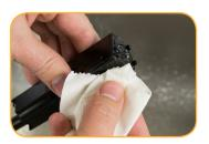
Wipe away excess solution. Soak in tap water for 15 minutes and calibrate.
