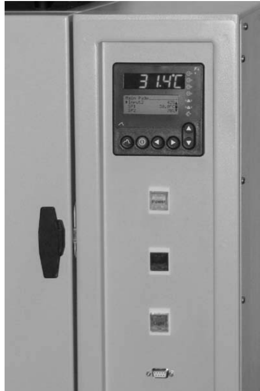
Figure 5-3 Controller and Pilot Lights
