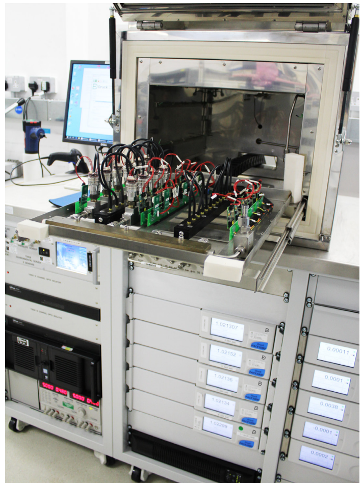
Picture 3: A typical Automated Production Test System
