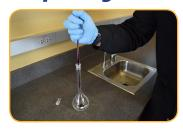
1. Start with a 2.5% Rhodamine WT solution. Pipette 1.0 mg/L of the solution into a 250 mL Class A volumetric flask.
