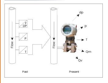
The Tek-Bar 3800 XA Multivariable Transmitter measures differential pressure, static pressure (absolute or gauge), and process temperature. It also performs flow calculations, compensating for pressure or temperature and accounting for variables such as discharge coefficient, thermal expansion, Reynolds number, and compressibility factor.
