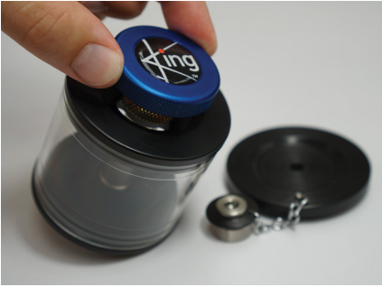
Fig. 5-1 Disassembly of hydraulic reservoir
