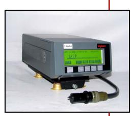
The EdgeTech Model 137 Vigilant Aircraft Hygrometer is a rugged, shock mounted military qualified instrument used for the primary measurement of dew point in flight or in installations with existing flow, such as wind tunnels.
