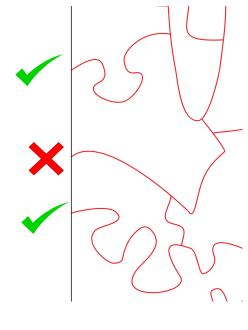
3. No sharp points. They must be rounded to prevent issues when laser cutting.
