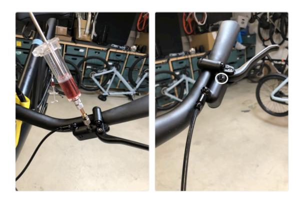
(i) When removing the syringe hold a cloth under the brake lever, because oil can leak out
