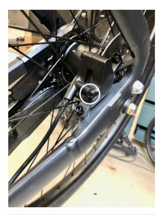
(i) You can prevent oil leaking on the brake pads and disc by covering up the parts with a cloth.
