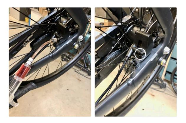
(i) You can prevent oil leaking on the brake pads and disc by covering up the parts with a cloth.
