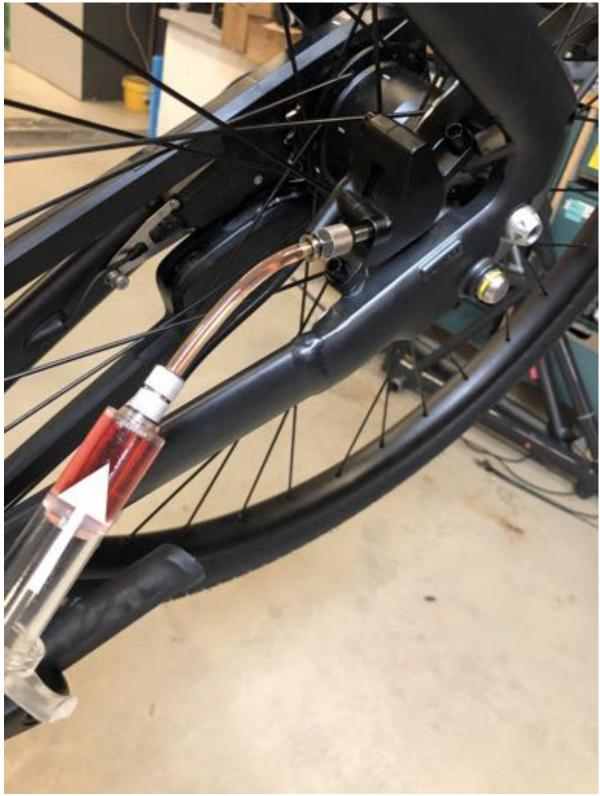
• When all air appears to be in the syringe by the brake lever, squeeze its fluid back into the system making sure to stop before the air re-enters.
