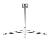
2. Fix the stand base to the stand body by tightening the screw.
