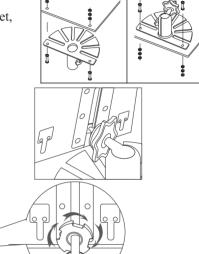
2. U-Bracket Installation (optional)1) Use the screw fixed the U-bracket. Put the monitor into the bracket, adjust angle and locking it.
