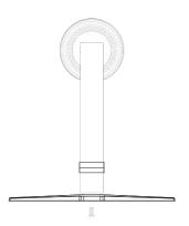
3. Attach the cover plate by pressing it onto the stand body.
