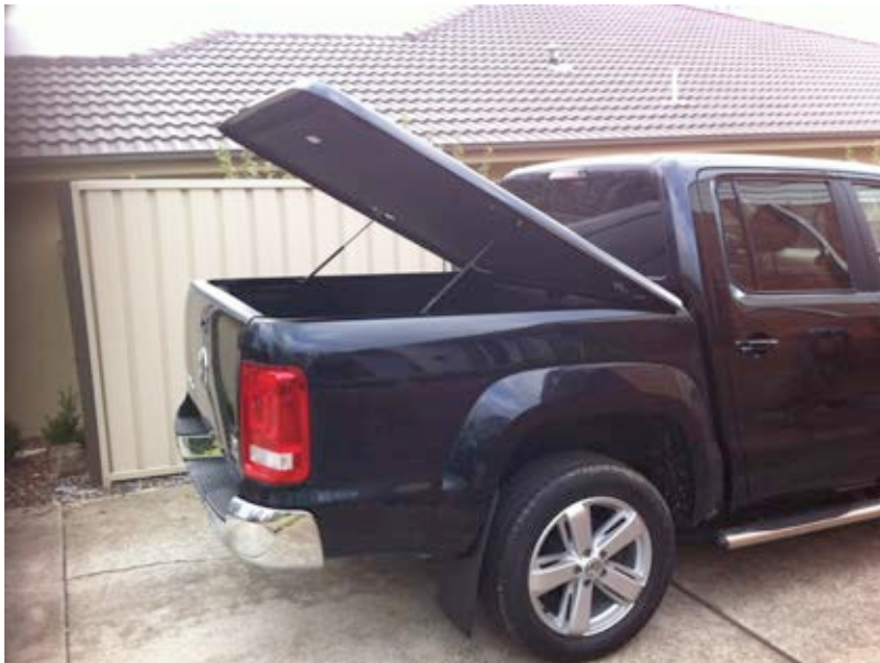
Lidlok auto remote servo , activated by key fob
