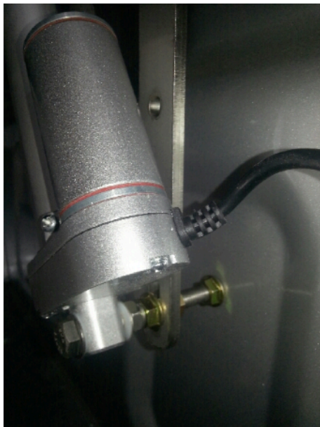
power strut bottom pivot if fitted.
