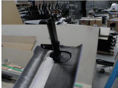
ranger Only bar attachment showing washer packing,
