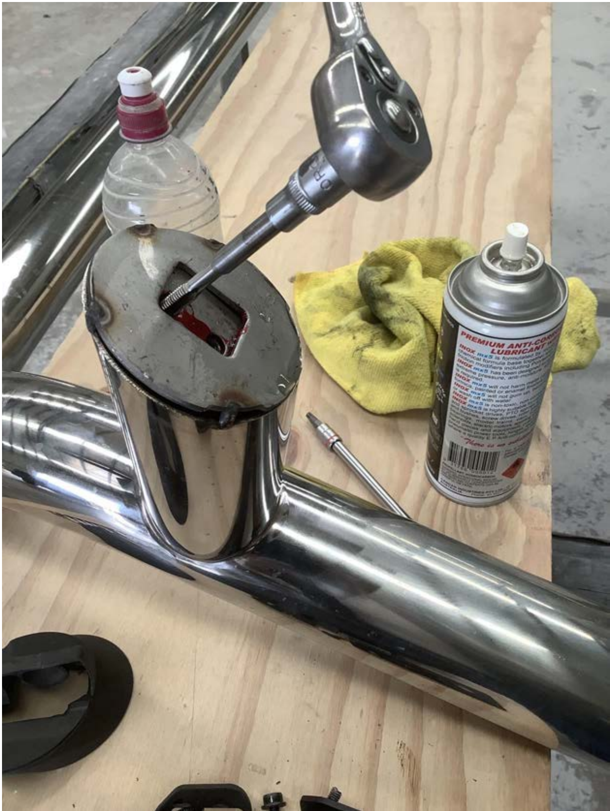
Trim boots and fit rubber seals. Fit sports bar to lid with 8 screws and washers. Fit pastic caps using silicone. Make sure to trim front leg boots to clear rectangular spacer blocks stuck on lid
