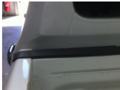
5. Lay foam tape across front edge of infil to sit on and seal
