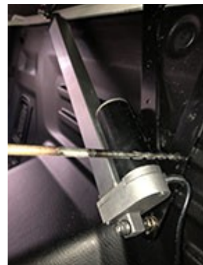
18. Drill 6.5mm hole through tub liner and inner panel
