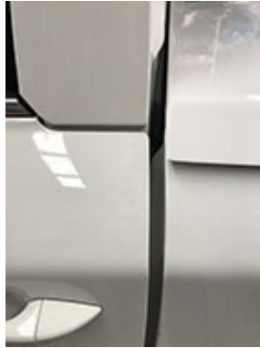
11. Align Lid with bodywork and with an even gap left to right
