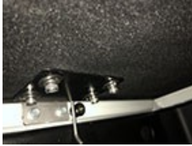
10. Put lid back on car and loosely fit hinge screws
