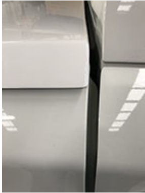
11. Align Lid with bodywork and with an even gap left to right
