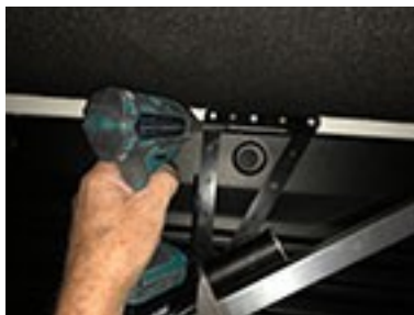
14. Swing up triangular bracket to side rail and screw in place
