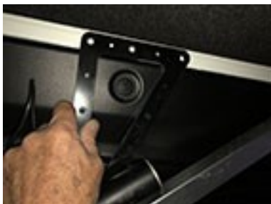
14. Swing up triangular bracket to side rail and screw in place
