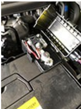
37. Connect power harness to battery
