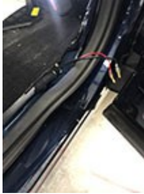
36. View of driver's floor with door seal panel removed and wire visible
