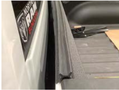
7. Stick seal to top of front wall, trim if necessary
