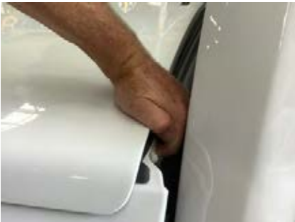
10. Check lid is centred on the car and not too tight over tailgate. Get another person to squeeze down on lid while you tighten hinge bolts
