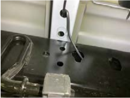
24. Connect power loom to battery and cable tie to loom across firewall to right hand side of car
