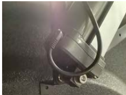
17. Fit self drilling hex screw to this hole
