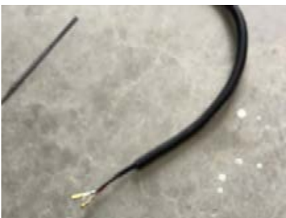
26. Fit wires from struts into corrugated power loom
