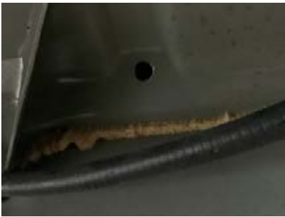
28. Carefully drill an 11mm hole from underneath the car.
