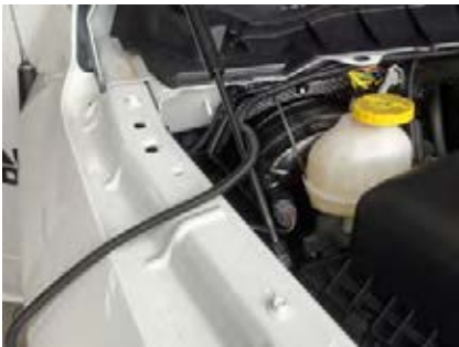
25. Bring power loom between inner guard and firewall to underneath the car
