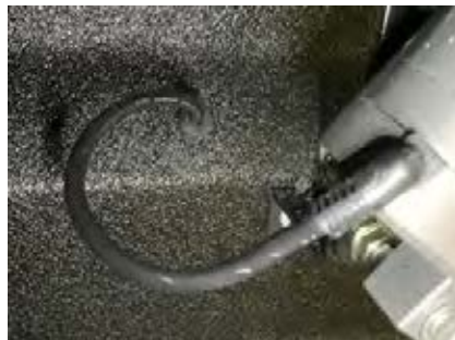
19. Fit strut wires through the hole and fit rubber grommet to hole , leave enough loose wire to allow for movement of strut
