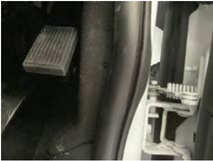
27. Remove drivers side sill panel two small screws behind door seal
