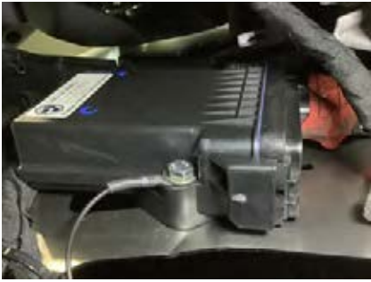
35. Connect earth wire to this bolt (under dash left of column)
