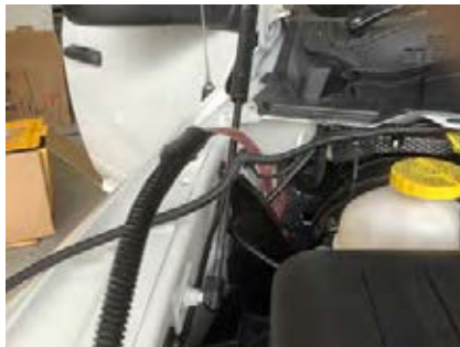
25. Bring power loom between inner guard and firewall to underneath the car
