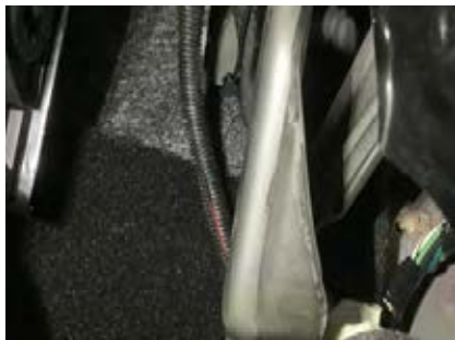
30. Bring the corrugated wires into the cabin and cable tie to the handbrake cable and follow to the underside of the dash
