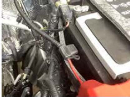
24. Connect power loom to battery and cable tie to loom across firewall to right hand side of car
