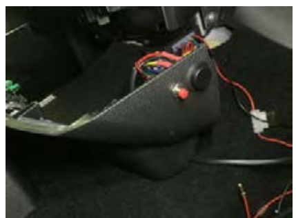
33. Fit red button and isolator switch to centre console trim and connect wires
