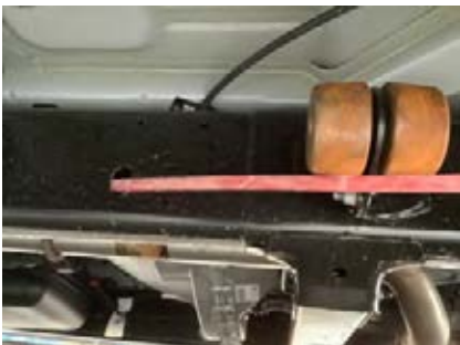
20. Bring wire from back through right hand chassis rail and out of the hole under the hand brake cable
