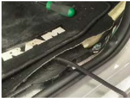
29. The hole will be behind the black plastic box so care must be taken when drilling not to hit the box.
