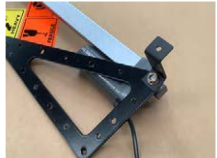
12. Fit 'Z' brackets to strut assemblies as shown
