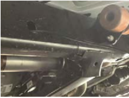
22. Wire from struts exiting chassis under drivers seat
