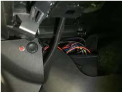
34. Stow control and wiring neatly, leave easy access to fuse
