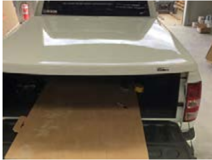
7. Stick seal to top of front wall, trim if necessary
