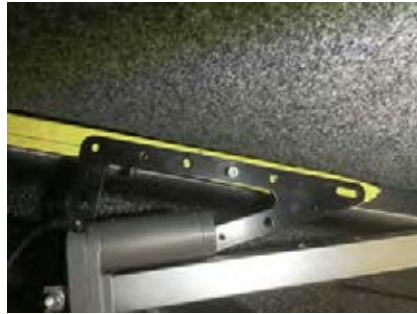
14. With tailgate open and lid in closed position bolt struts to the lid with the struts in the closed position and mark hole positions along 17 mm line
