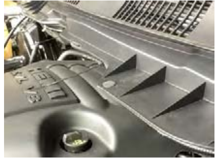
24. Connect power loom to battery and cable tie to loom across firewall to right hand side of car
