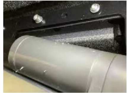
15. Fit button head screw in the hole above the electric motor
