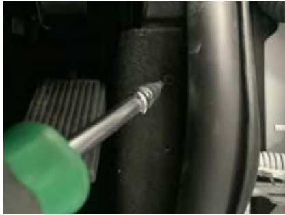
27. Remove drivers side sill panel two small screws behind door seal
