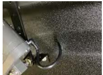
19. Fit strut wires through the hole and fit rubber grommet to hole , leave enough loose wire to allow for movement of strut
