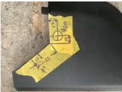
36. Red button and isolator switch locations for this panel
