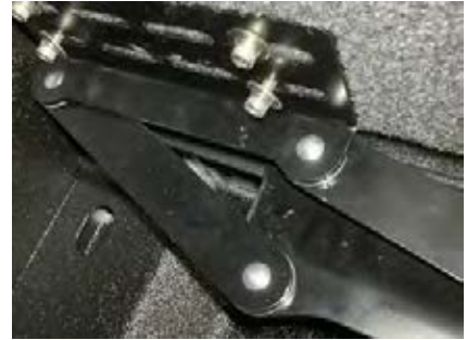
9. Fit hinge bolts loosely. 6x20 shcs 6mm spring washers and 1/4x3/4 flat washers
