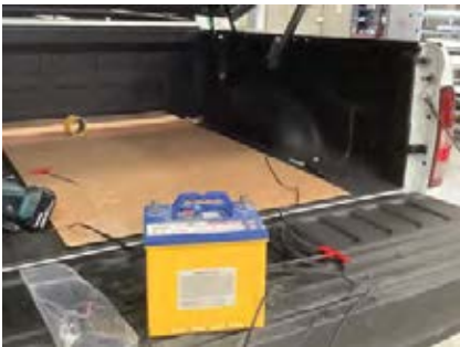
16. Temporarily connect struts to loom and open lid using 12v power source
