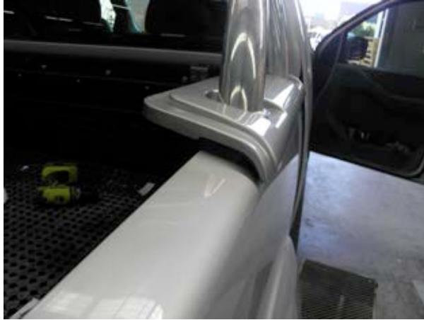
STX with packer to allow over lip tub liner to be inserted underneath
