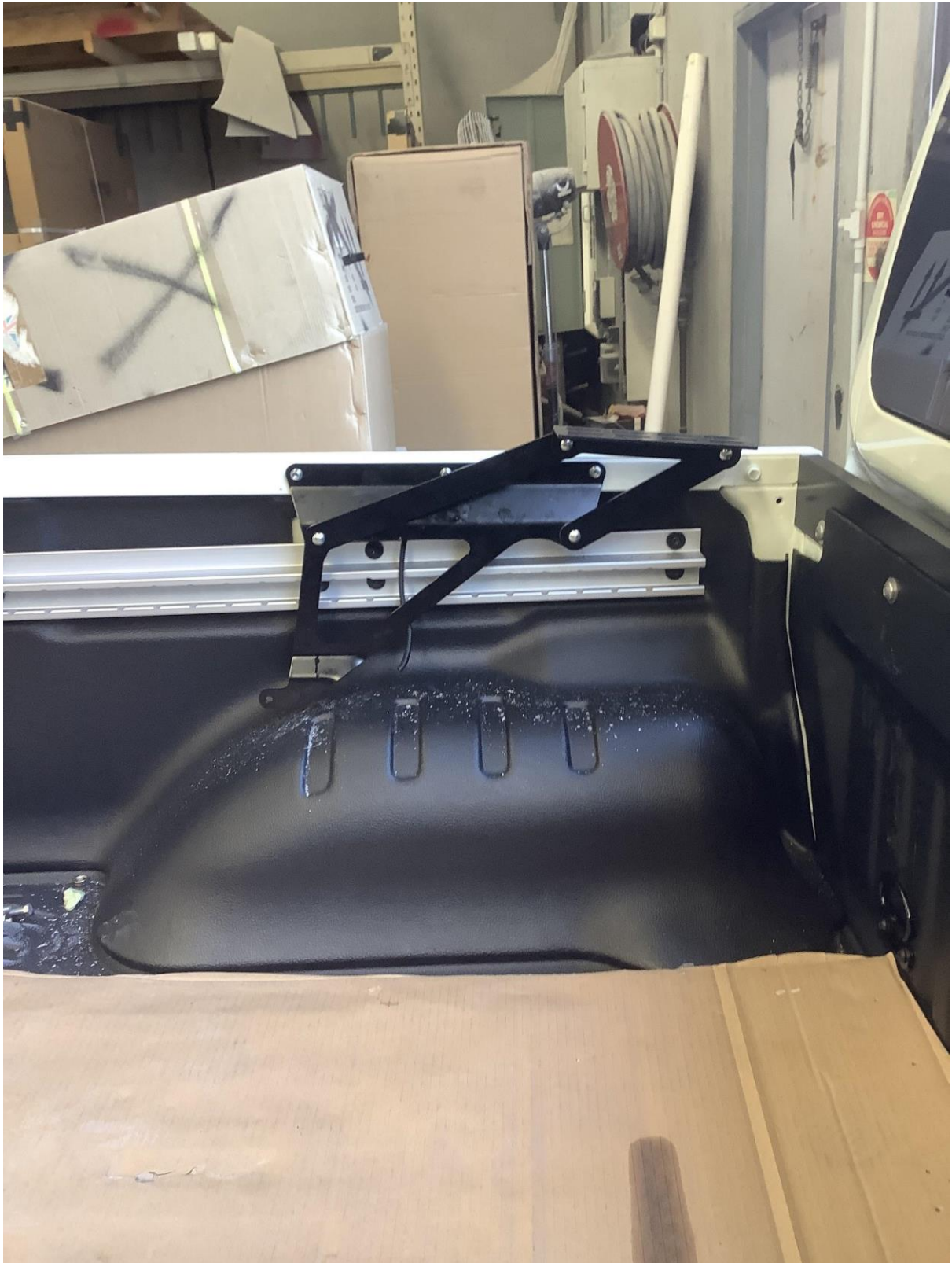
Drill 9 mm holes and fit nutserts and mount hinges
