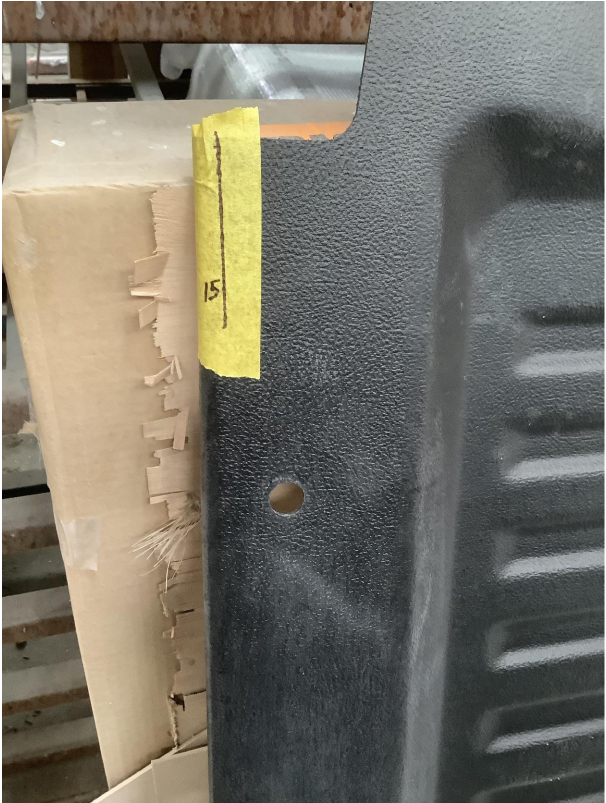
Trim 15 mm off top edge of front wall tub liner
