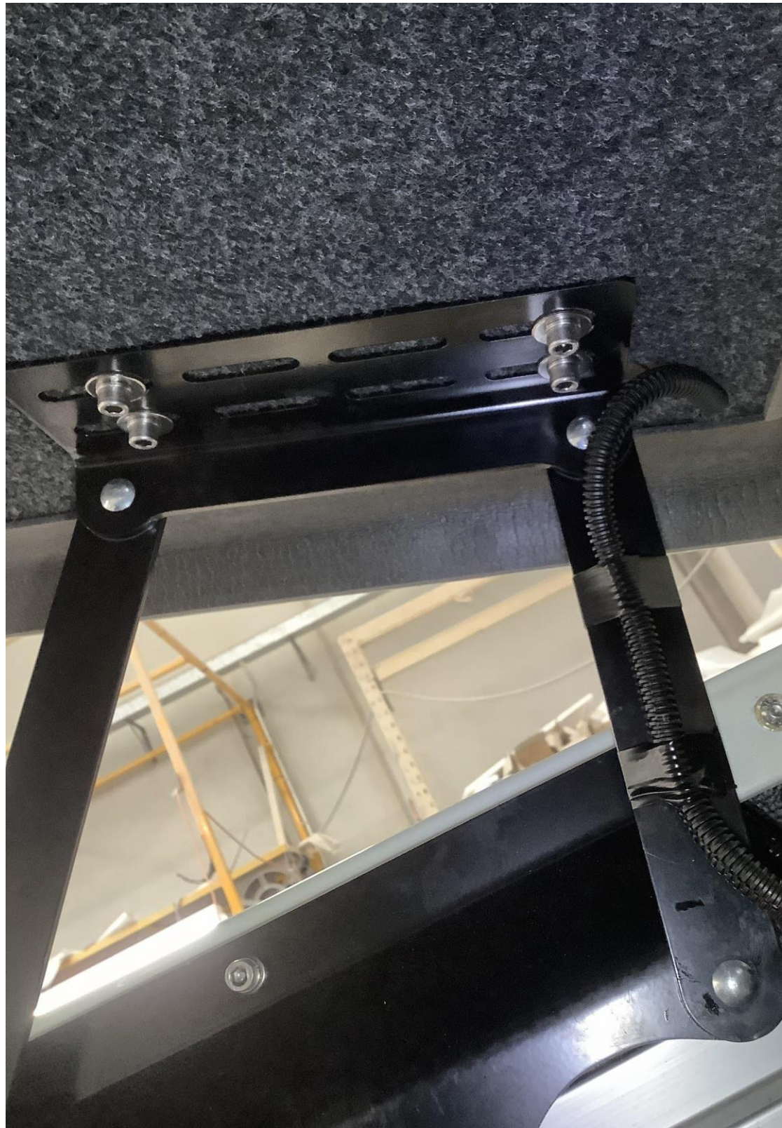
Connect and tape brake light wires to hinge arm allowing enough slack for movement of the hinge
