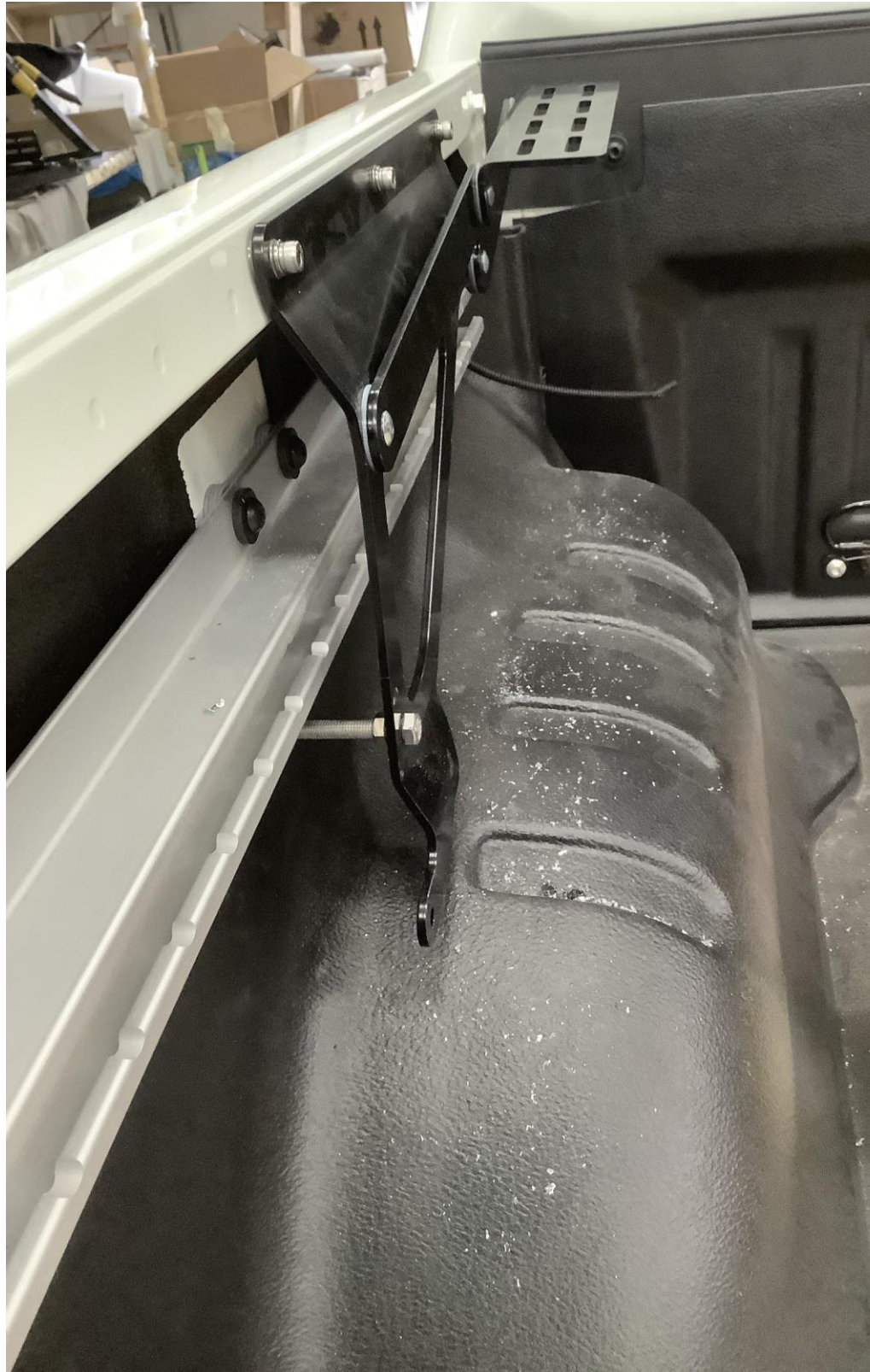
Fit 8 mm set screw and nut and screw in till bracket is verticle and then tighten gold nut
