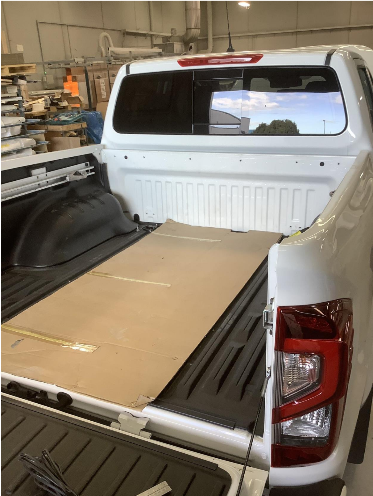
Remove sports bar and brackets. Remove front wall tub liner.
