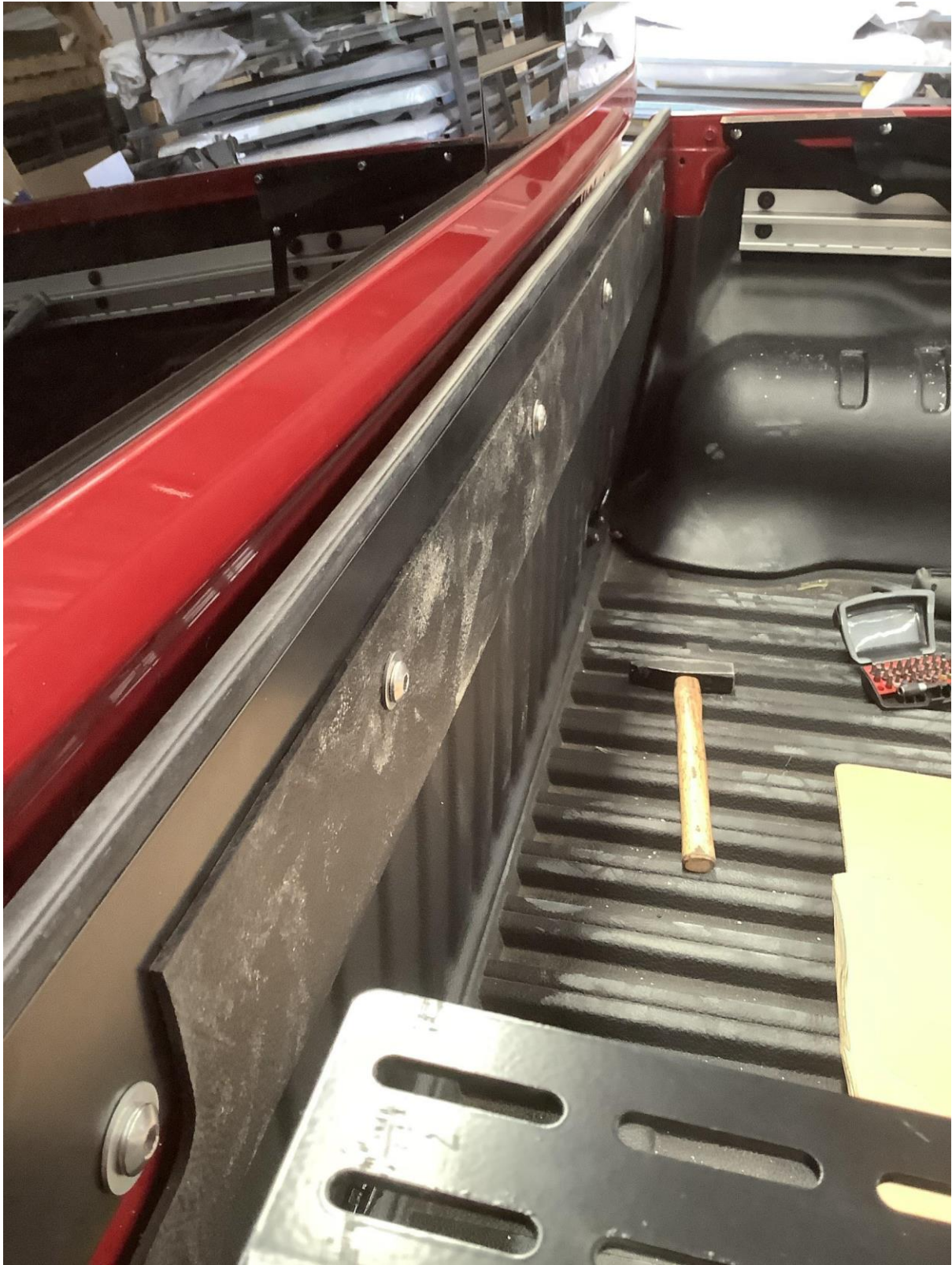
fit infil panel to front wall and refit tub liner panel.(trim raised seal from left and right sides of front wall so that infil panel sits flat)
