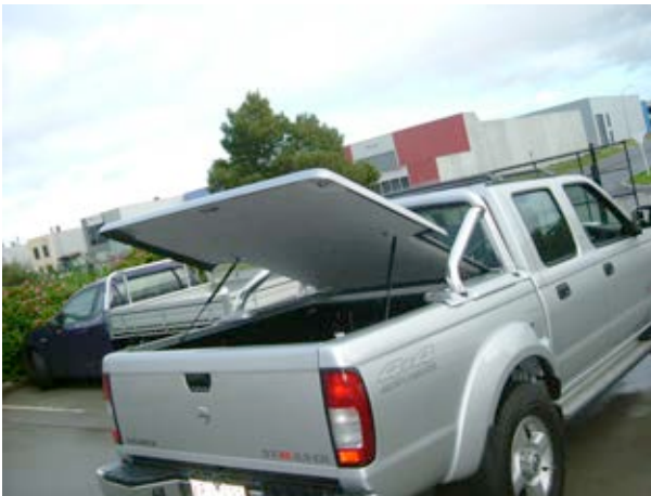
note strut mounting position Cylinder barrels upper! Rods Lower.
